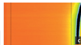
c. Resistivity map of multi-crystalline Si brick
